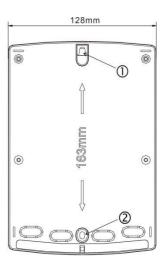
Size of controller for electrical heater of 3000W
