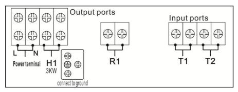
➤ **Power terminal N, L**: AC220V, 20A, for power connection, L: live wire, N: zero wire, protective wire, please connect to ground reliably.
